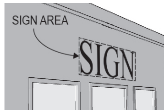
Figure 9-3 Wall Sign without panel
